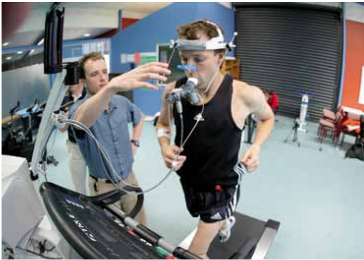
Figure 5.39: An athlete undertaking a treadmill test for maximal oxygen uptake
